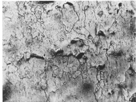
Figure 6 DS lead A stressed at 2 \times 10^3 lb/in. 2 . Chemically polished after failure at 16.8%. Area showing intercrystalline cavities and grain elongation ( \times 280 ).
